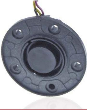
The ultrasonic level sensor MOTOSONIC generates a high frequency sound wave to measure the time, the wave needs to run to the fluid level and back, after it was reflected by the liquid surface. Based on the measured time and the speed of sound, the distance between the sensor and the liquid surface can be calculated, and by this means the tank content as well.
